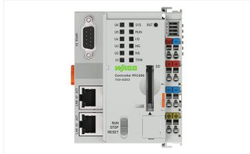
The PFC300 Controller is a compact PLC for the modular WAGO I/O System. Besides network and fieldbus interfaces, the controller supports all digital, analog and specialty modules found within the 750/753 Series.
