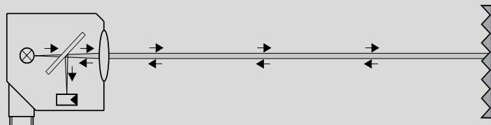
With photoelectric retro-reflective sensors one speaks of the autocollimation principle when the light reflected from the reflector travels parallel to itself (i.e. within itself). The light emitted by the sensor hits a reflector and is reflected. The reflected light is then deflected to a receiver by a semi-transparent mirror and evaluated.
