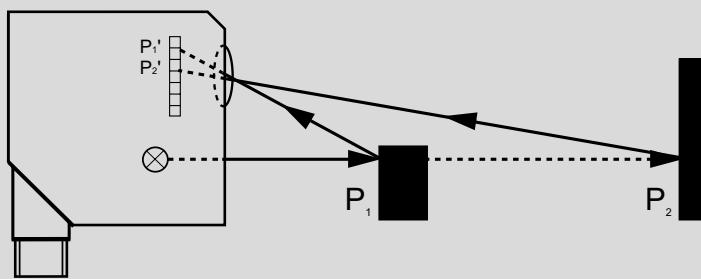
In the case of fixed background suppression, the transmitter and receiver elements are fixed-mounted. The operating range is defined by the overlapping of the transmitter and receiver angles. Objects outside this operating range cannot be detected.
